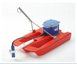
This integrated Thurn system is available with a turn-key single beam and side scan solution for autonomous or remote-controlled collection of depth and sonar imagery. Using single frequency or dual frequency echosounders, the Imagenex yellowfin OEM side scan and an SBG 3rd generation dual-antenna motion and positioning sensor.
